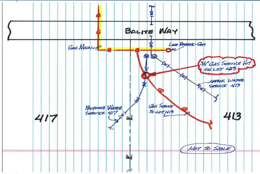
The water valves were in the same box. The dig ticket was for a locate at 417. The service to 413 passed between 417 and the water box. The locate was accurate for the dig ticket. The excavator did not know that the water valve for 417 was on the property of 413.
