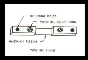
• A precisely calibrated resistor designed to drop 50 MV when the rated current flows through it.
