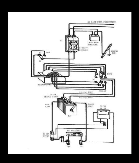
Power Train consist of a transformer and a stack.
