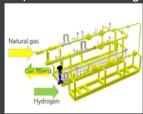
Blending skid for hydrogen blending in natural gas fuel supplies to industrial processes.
