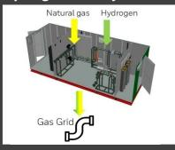
Compact hydrogen injection system for green or blue hydrogen entry to natural gas grids.
